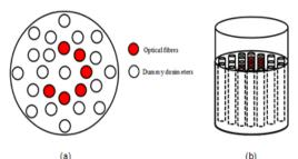
Figure 1. (a) The top view of Gammacell chamber with samples and dummy dosimeters. (b) The side view of Gammacell chamber
